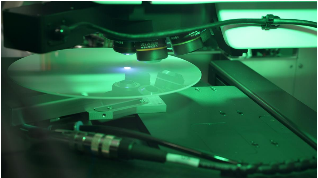
Figure 1. Sapphire wafer under an MX series microscope. Image courtesy of PVA SPA.
